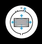
Cylinder flooded under vacuum 2. with Tanalith E wood preservative and the addition of Tanatone brown colourant, if required.
