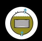
Hydraulic pressure applied, forc-3. ing the preservative deep into the structure of the timber. The amount of penetration achieved is a function of species treated and treatment specification.
